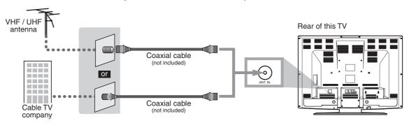
\*Once connections are completed, turn on the TV and begin initial setup. Channel scanning is necessary for the TV to memorize all available channels in your area. (Refer to "INITIAL SETUP" on page 12.)
